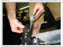
Step 18: Slide Lead Screw Assembly Out from the Rear of the Track
