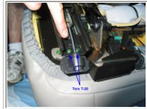
Step 14: Remove Two Torx T-20 Screws Near the Front of the Seat Track
